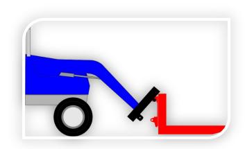
With your tractor, tip the connection harness toward the ground (As if you were emptying a bucket). Lower the loader and bring the tractor harness against your ALO implement.
