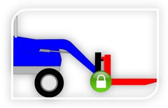
two. Then engage the latches on the tractor harness to lock your ALO implement in place.
