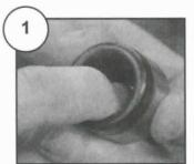
Smear grease into bearings and check for dirt.
