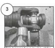
Grip loosened cup in vise, strike yoke arm to drive yoke off cup. Repeat on opposite cup.
