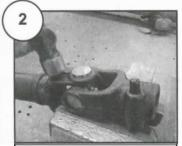
Position joint in loose vice, strike top arm of unsupported yoke to drive the top cup up. Repeat on opposite side.
