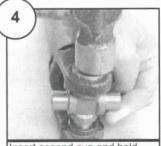
insert second cup and hold cross into cup. Drive cup flush with arm.
